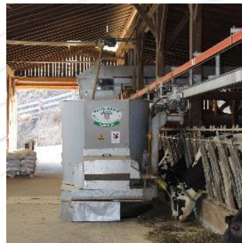
Example of Automatic feeding systems (AFS) fully electric powered
