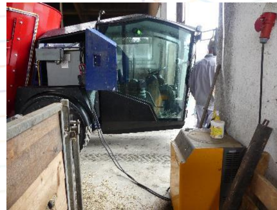
Example of self propelled electric powered mixer wagon (18+15 kW engines power)
