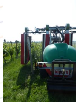
Sprayer with recovery systems capable to reduce until 80% the product distributed
