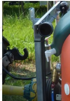
Kit of reader of dead plants and rows for selective spraying
